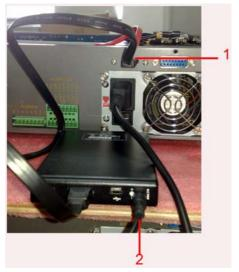
Fig. A-1 Portable Hard Drive Connection 1. Data cable connecting with E-SATA jack
